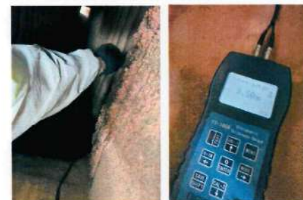
Primary Supper Heat Tube Thickness Check
