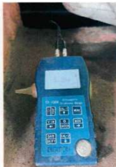
Secondary Supper Heat Tube Thickness Check
